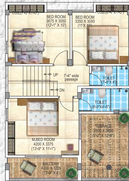
FIRST FLOOR PLAN
